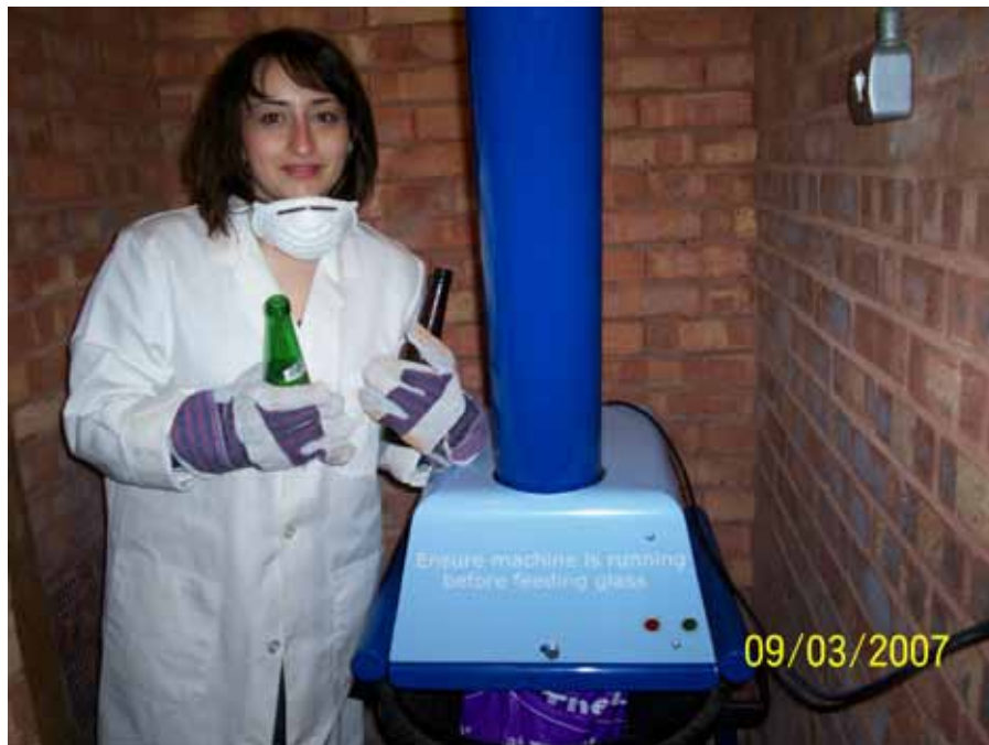
Granulating glass by the imploder at UoB workshop. Miss Thomi Argyroudi, MSc Civil Engineering student, March 2007
