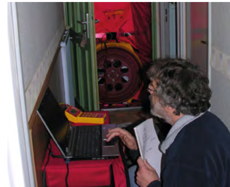
A Blower-door test in Outreau (January 2013).
