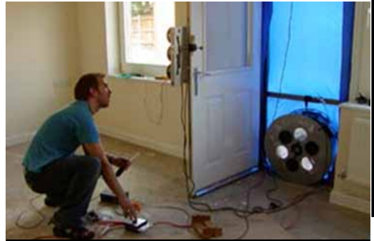
Ryan Southall carrying out a pressure test, using a 'blower' door, to determine the level of air-tightness of the building.
