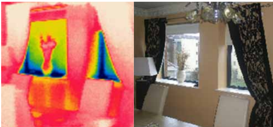
Thermographic image illustrating the relative temperatures of interior surfaces and a photo for comparison.
